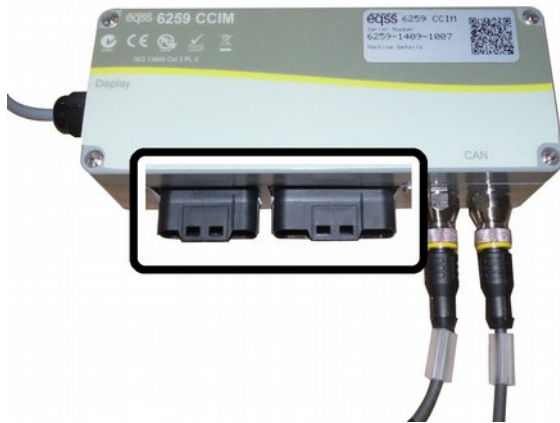
Illustration 1: CCIM Bulkhead Connectors Removed
