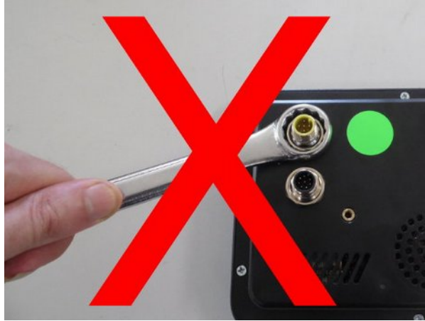
Illustration 6: Do Not Over Tighten Nuts
