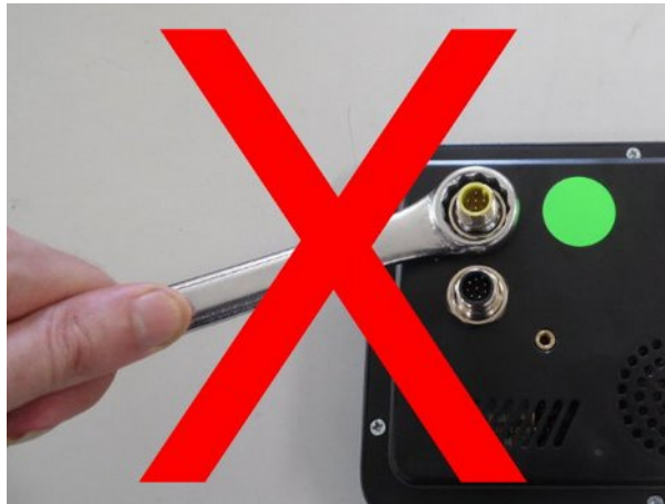
Illustration 6: Do Not Over Tighten Nuts
