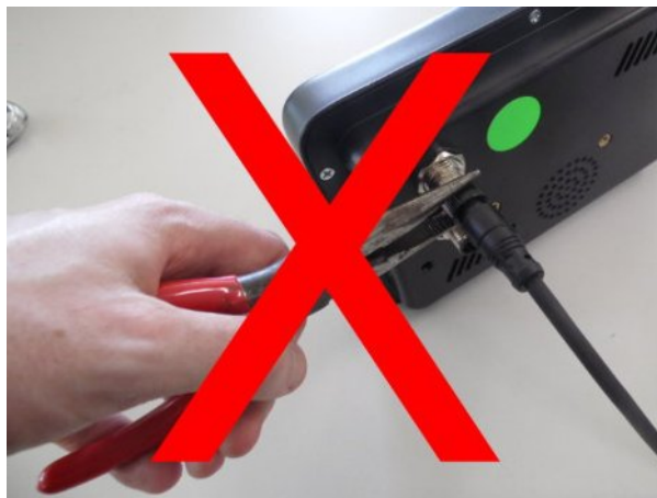
Illustration 5: Do Not Use Tools To Tighten Connector
