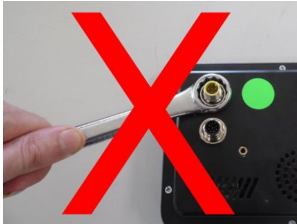
Illustration 6: Do Not Over Tighten Nuts
