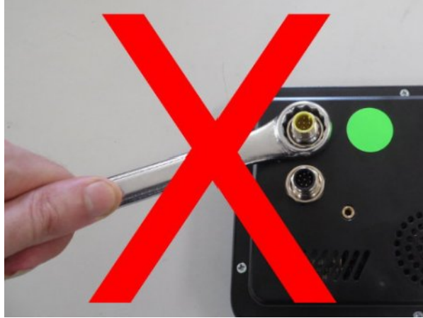
Illustration 7: Do Not Over Tighten Nuts
