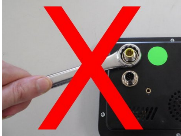
Illustration 7: Do Not Over Tighten Nuts
