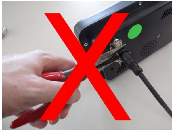
Illustration 6: Do Not Use Tools To Tighten Connector
