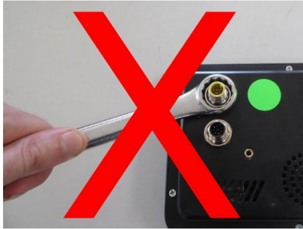
Illustration 7: Do Not Over Tighten Nuts
