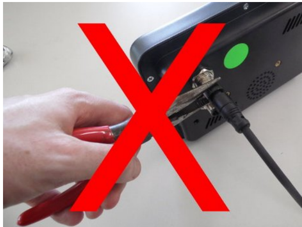
Illustration 5: Do Not Use Tools To Tighten Connector
