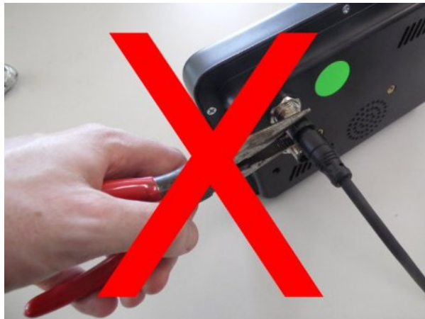
Illustration 6: Do Not Use Tools To Tighten Connector
