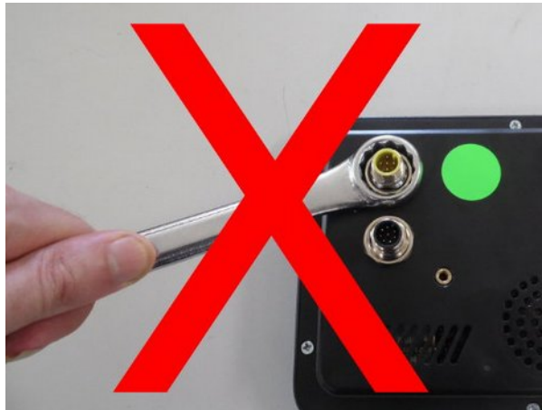
Illustration 6: Do Not Over Tighten Nuts
