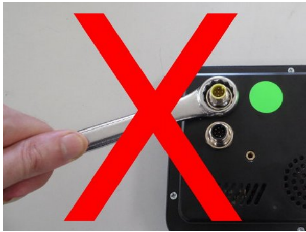
Illustration 6: Do Not Over Tighten Nuts
