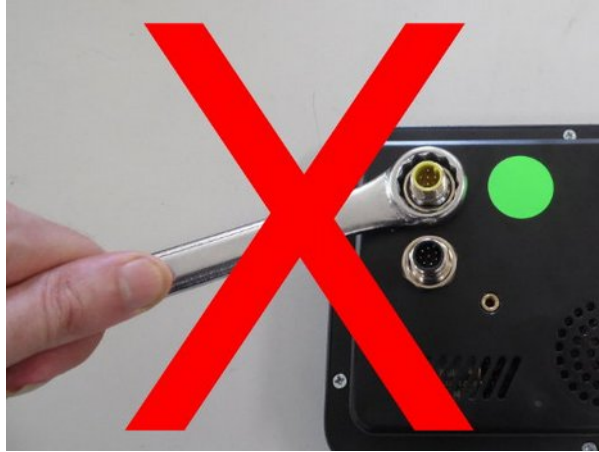
Illustration 6: Do Not Over Tighten Nuts
