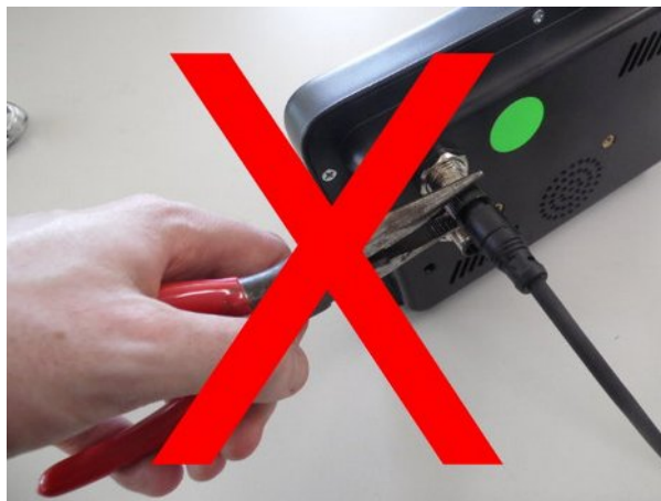
Illustration 5: Do Not Use Tools To Tighten Connector
