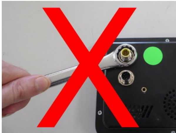
Illustration 6: Do Not Over Tighten Nuts
