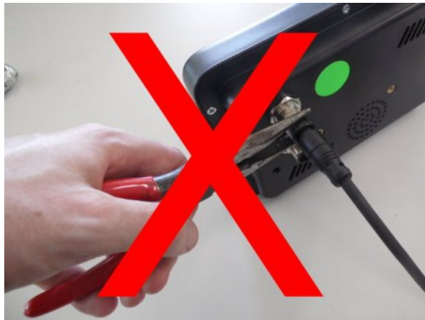
Illustration 5: Do Not Use Tools To Tighten Connector
