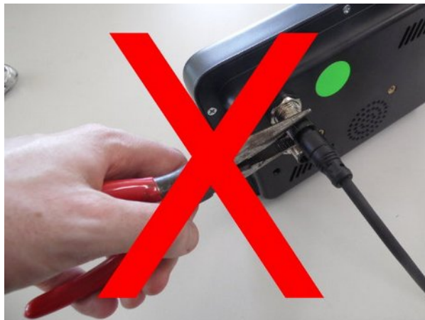
Illustration 3: Do Not Use Tools To Tighten Connector
