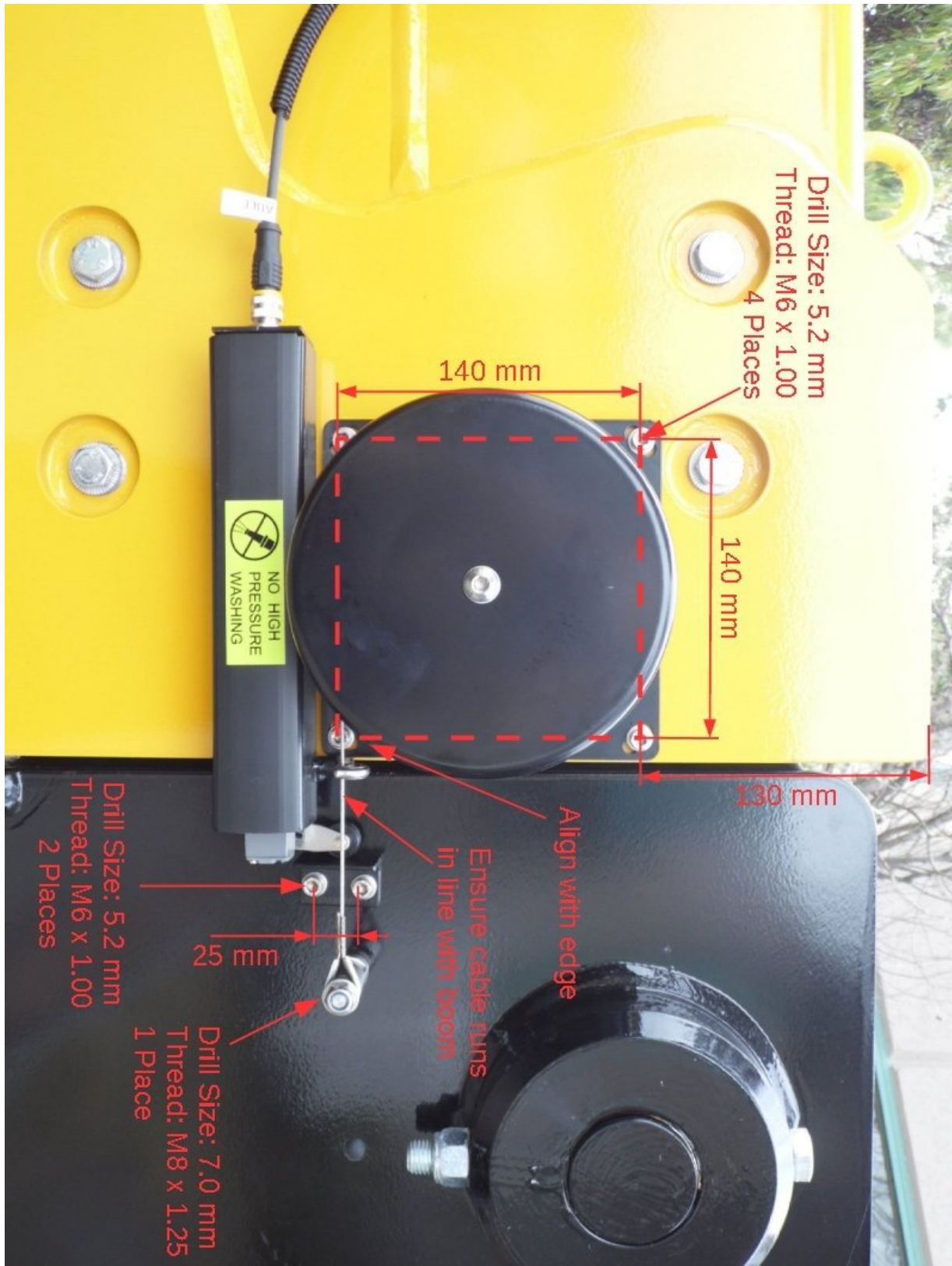
Illustration 3: Cable Reeler Mounting Position
