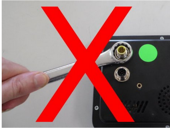
Illustration 4: Do Not Over Tighten Nuts
