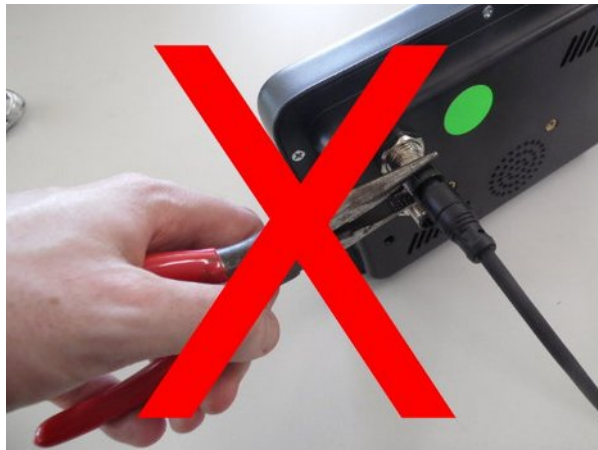
Illustration 3: Do Not Use Tools To Tighten Connector
