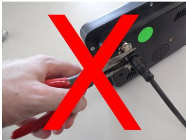
Illustration 5: Do Not Use Tools To Tighten Connector
