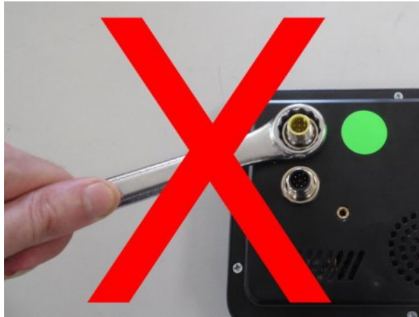
Illustration 6: Do Not Over Tighten Nuts
