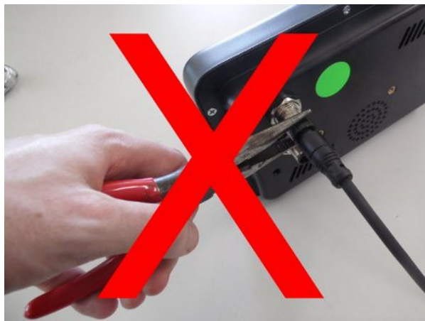
Illustration 3: Do Not Use Tools To Tighten Connector
