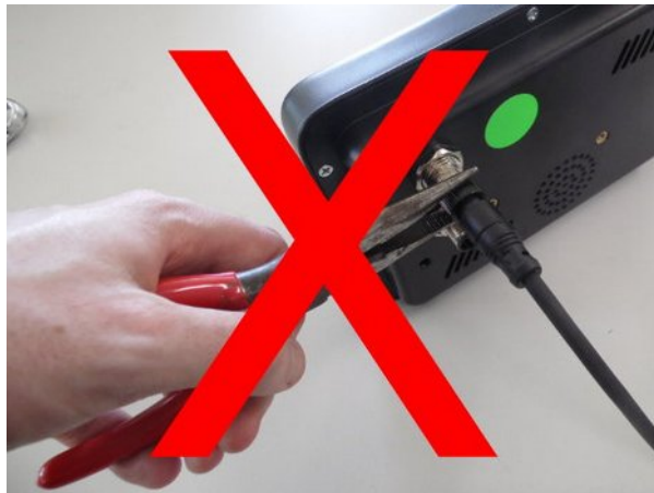
Illustration 5: Do Not Use Tools To Tighten Connector
