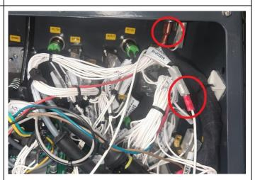
8. Mount the OverWatch ECU inside the control box using the adhesive velcro tape.
