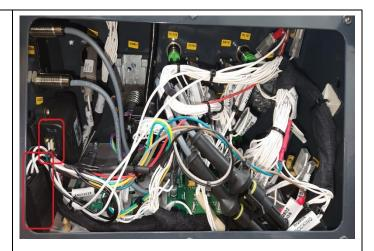
10. Re-attach the bottom plate to the control box. Secure the operator sensor cable by using a p-clip as shown in the image. After installation, power the machine for platform controls and press the emergency stop.
