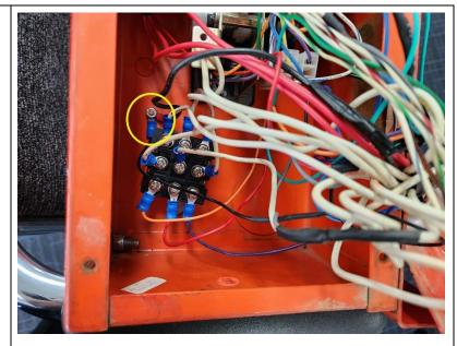
13. Connect the 8-Pin connector from the operator sensor and the 12-Pin connector from the OverWatch harness, into the ECU module.
