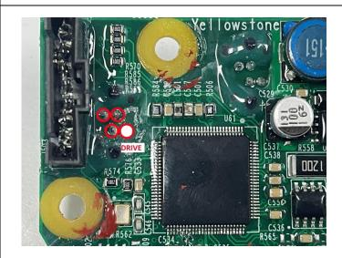
8. Trim down the two **Horn** signal pins. These pins are located as displayed in the adjacent image. Using a fine pair of side cutters make sure that the pins are trimmed flat.
