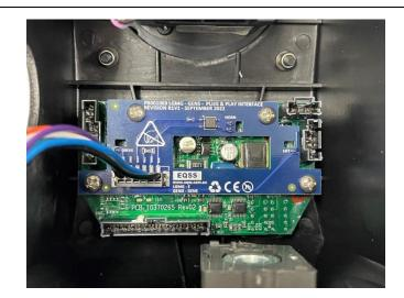
11. Install the Overwatch joystick connectors in between the joystick and the control box circuit board.
