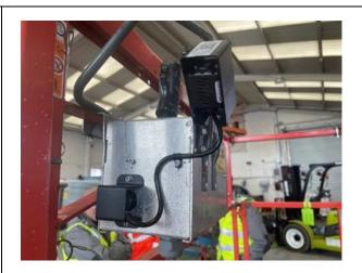
6. Drill a **20mm** hole to run the operator sensor M20 cable gland and drill two **5.2mm** holes for the cable gland guard.
